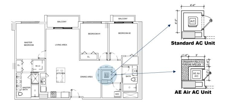
Look at the value of the now usable space by installing HydroTech Slim 16 **-vs-** a standard size water source heat Pump
